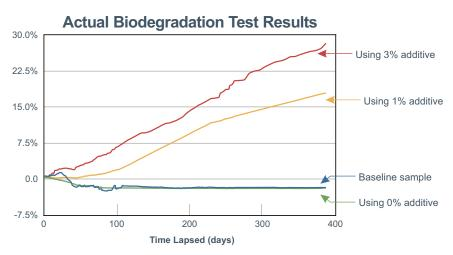
Independent lab results using ASTM D5511 method indicate an accelerated path of biodegradation for plastic samples manufactured by Elevate Solutions Group. Those made with a 3% additive biodegraded 28.3% within 387 days. And those using just 1% additive biodegraded 17.9% within 387 days. Actual results may vary depending on landfill conditions. Methane gas created from the biodegradation process can be captured and converted into energy where facilities exist.
